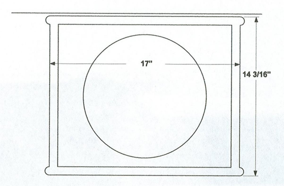
THE BOX IS GLUED INTO A 1/4" DEEP x 3/4" WIDE DADO CUT INTO THE BAFFLE.
