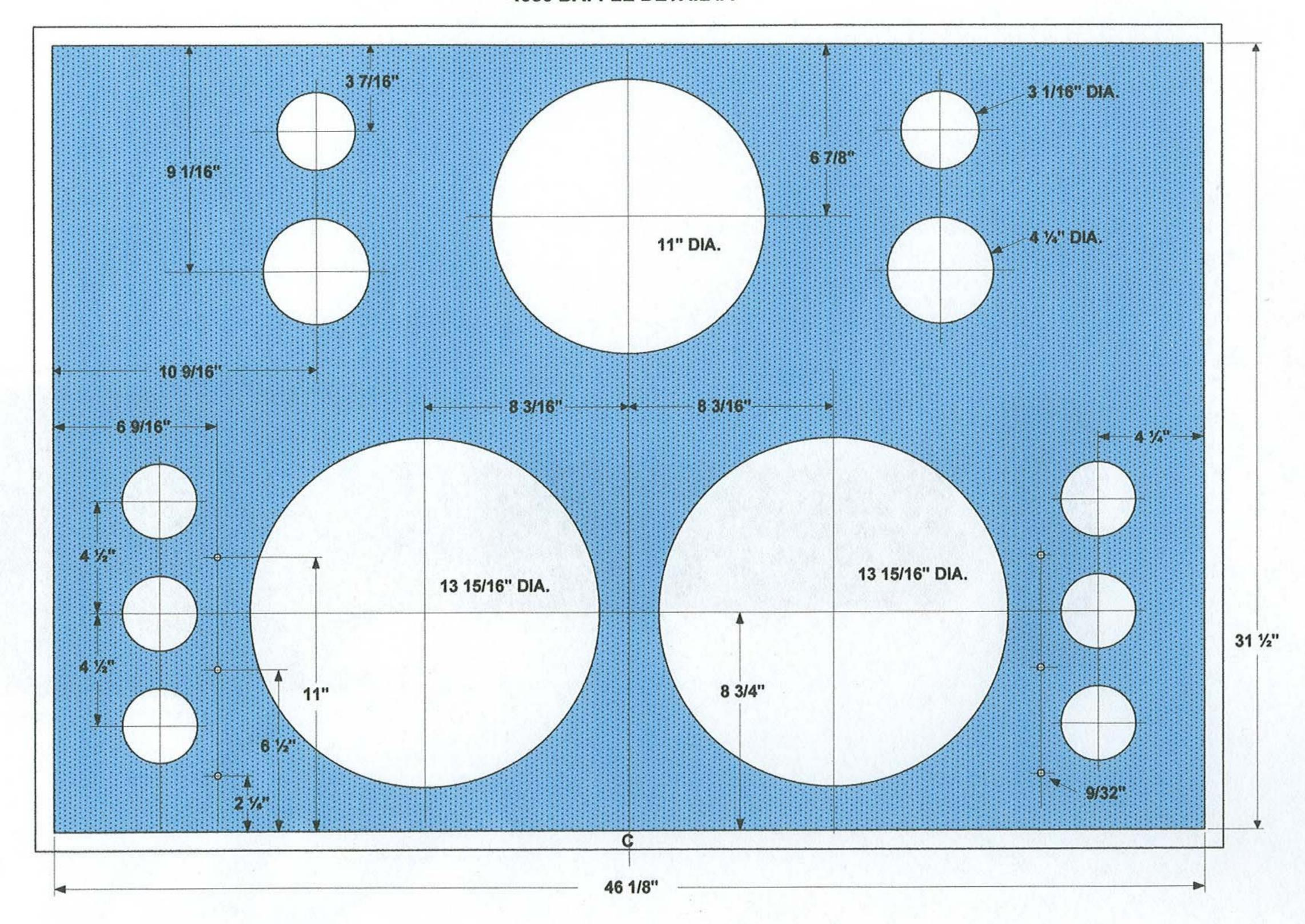
THE BAFFLE LAYOUT AND LOCATION OF ALL HOLES IS ESSENTIALLY THE SAME FOR ALL MODELS, EARLY TO LATE, INCLUDING THE 4350B. EXACT LOCATION OF EACH CUTOUT MAY VARY 1/16" FROM CABINET TO CABINET. THIS STATEMENT IS BASED ON MY OBSERVATIONS OF 6 TO 8 PAIRS OF ORIGINAL CABINETS.
