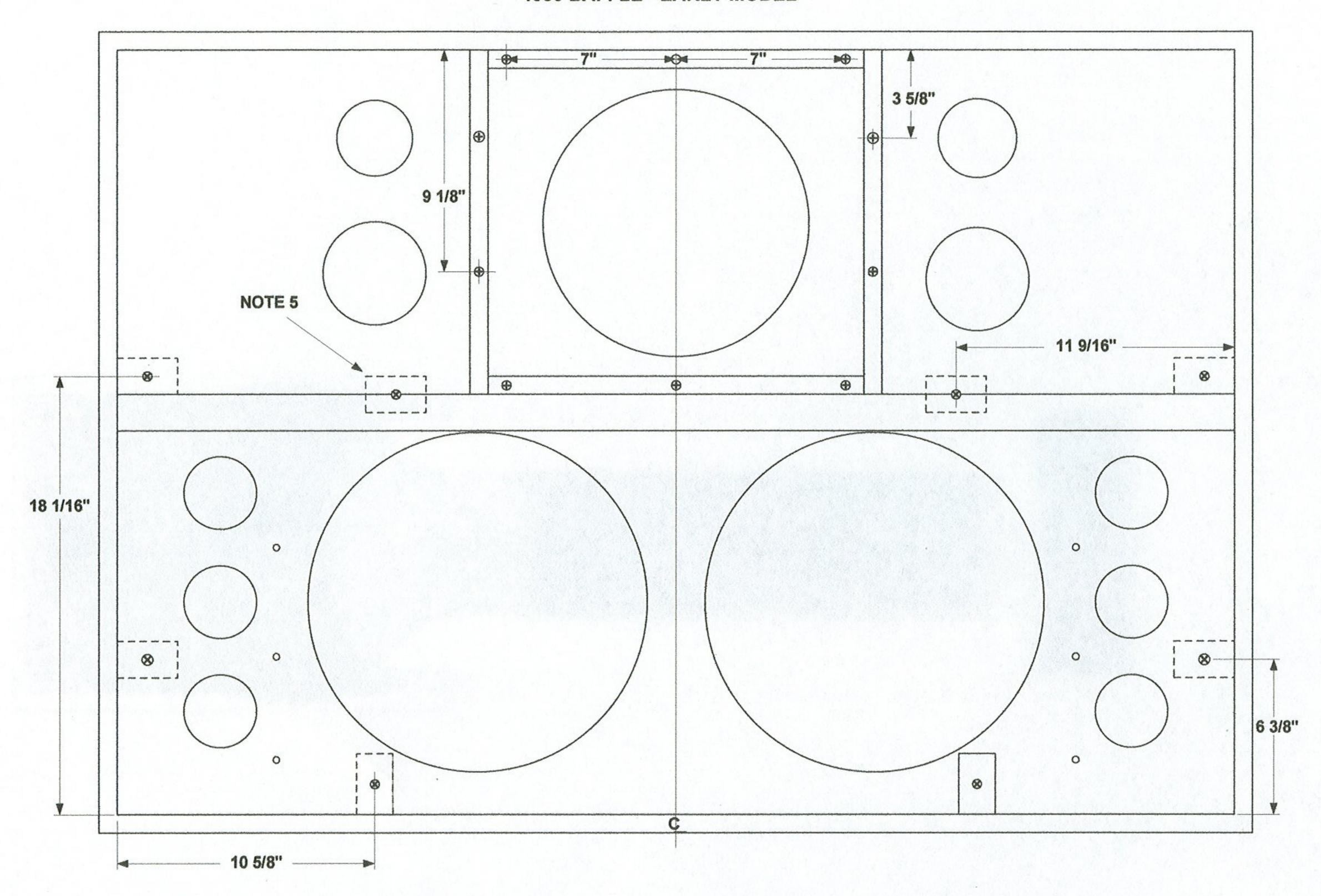
EARLY MODELS HAD ALL BRACES SCREWED FROM THE OUTSIDE -BAFFLE AND BACK. SCREW HEADS ARE VISIBLE ON THE BAFFLE AND BACK. SCREWS USED WERE #8 2" PHILLIPS HEAD
